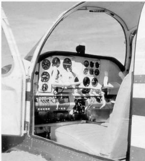
Above: The Aircruiser's front cabin and instrument panel showing its control wheels and high standard of interior finish for a prototype. Millicer Family
